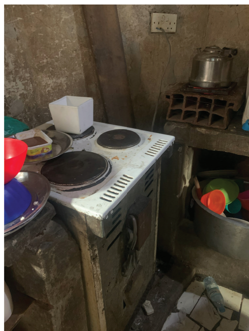
Photo caption: A damaged electric stove which a woman had stopped using because it was shocking her and her children (left). An example of electric cooking with cooking coils (right). Photos by Jess Kersey and Judith Mbabazi.
