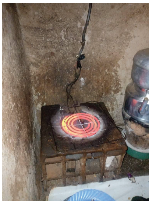
Photo caption: A damaged electric stove which a woman had stopped using because it was shocking her and her children (left). An example of electric cooking with cooking coils (right). Photos by Jess Kersey and Judith Mbabazi.
